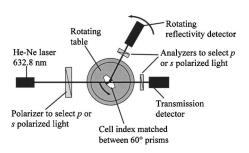
FIG. 1. Experimental arrangement of the time-resolved fully leaky guided-mode technique. The application of the voltage pulse from a function generator and the data collection at the transmission and reflectivity detectors are synchronized and controlled through a LABVIEW interface.
