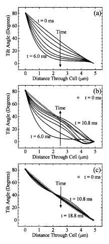
FIG. 3. The tilt profiles (with the tilt angle measured from the normal to the cell substrate) recorded during the application of the multiple-frequency pulse shown in Fig. 2: (a) during the application of the 2 kHz in 1 ms steps, (b) during the application of the 64 kHz pulse in 0.8 ms steps, and (c) with the voltage removed in 2 ms steps. In (b) and (c) the initial director profile at t=0 ms is shown for reference.
