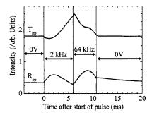
FIG. 2. Variation of optical intensity with time for transmitted and reflected p-polarized conserving data at a 74° angle of incidence. The data were collected on a 2  $\mu s$  time scale during the application of a 20  $V_{pp}$  multiplefrequency sinusoidal pulse as indicated.
