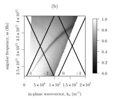
Fig. 3. TE polarized reflectivity as a function of in-plane wavevector and angular frequency, mapping the SPP dispersion on a zig-zag grating. (a) Numerical prediction and (b) measured data. Solid lines show the positions of diffracted light lights scattered by  $m\mathbf{k}_{gx}$ , where m=-1,+2,0,+3.
