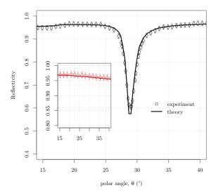
Fig. 2. Specular reflectivity of TE (black) and TM (red) polarized light as a function of polar angle,  $\theta$ , with a wavelength of 632.8 nm,  $\phi = 0^{\circ}$ . Circles: recorded data with error bars of 1%, line: fitted numerical model prediction.
