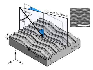
Fig. 1. The coordinate system of a zig-zag grating. The experimental sample parameters were  $\lambda_{gx} = 600 \text{ nm}$ ,  $\lambda_{gy} = 150 \text{ nm}$ , d = 29.9 nm with all measurements in this letter recorded at  $\phi = 0^{\circ}$ . Inset: A scanning electron micrograph of a replicated zig-zag surface in a polymer. (scale bar = 600 nm.)
