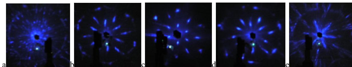
Figure 7. Characteristic blue laser ( \lambda=325\text{nm} ) diffraction patterns recorded in reflection from monolayers of 390nm spheres self-assembled at different pH factor of water. From left to right: pH = 2.8, 3.7, 4.1, 4.9 and 5.5. The size of the laser spot is approximately 3mm.
