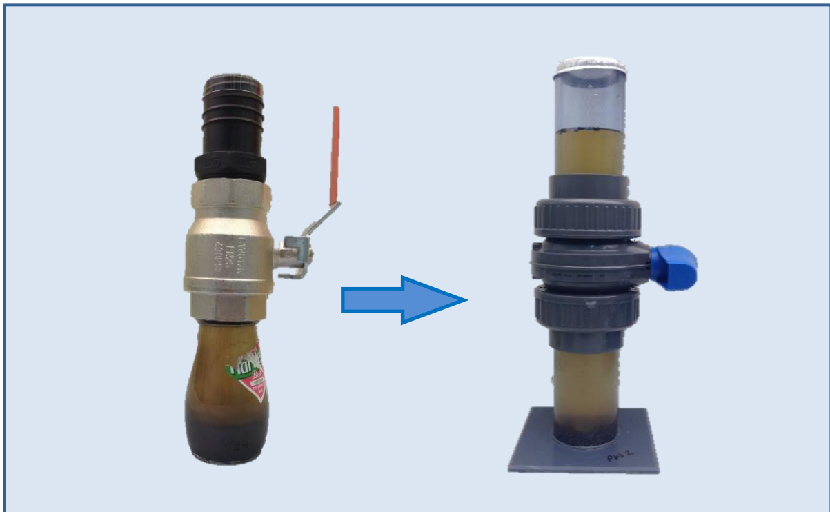
Figure 5.1. Sediment-Microplastic Isolation (SMI) unit, from first prototype to finished design.
