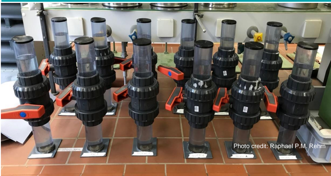
Figure 5.3. (a) Graphical demonstration of the SMI unit process and results and (b) an 'Army' of SMI units at the University of Augsburg, Germany investigating microplastic behaviour in soil erosion and run-off.
