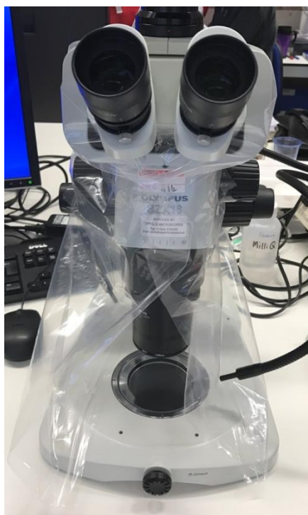
Figure SI 3.1. Additional contamination control when not using laminar flow cabinet.
