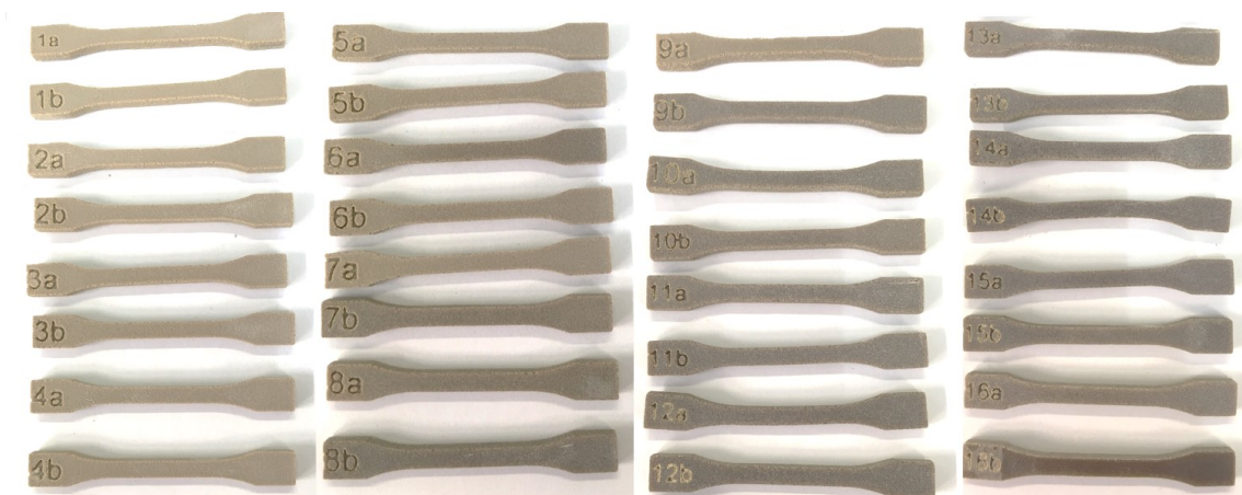
Fig. 9.6 Specimens removed from the cake, cleaned, and sandblasted. Note the change in color with cooling time. The specimens of lighter color remained cooling in the system for a longer time; therefore, they are more crystalline. In contrast, the darker specimens are less crystalline due to the shorter cooling time.
