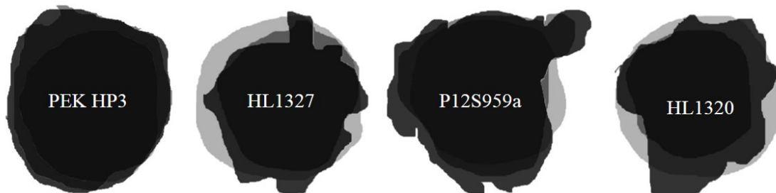
Fig. 5.5 Particle change with temperature. The darkest image corresponds to the particle at room temperature, followed by the image at (T), whilst the lightest colour corresponds to the particle at the maximum experimental temperature.
