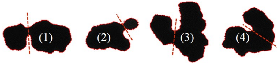
Fig. 10.5 Images of semi-sintered particles from the processed cake at (1-2) 265 °C and (3-4) 286 °C. The dashed lines represent the assumed partial sintering region between particles in the processed powder.
