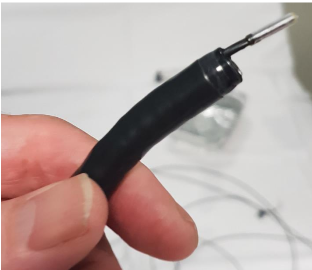
Figure 1-17 Examples of fibre optic probes capable of Raman Spectroscopy measurement in a clinical setting for cancer diagnosis, or application to in vivo surgical guidance to provide IMA, images Authors own.
