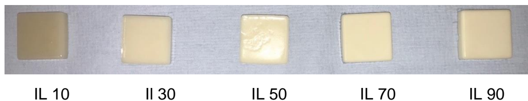
Figure 2-3 Photograph of complex gelatine phantoms with increasing concentrations of intralipid
