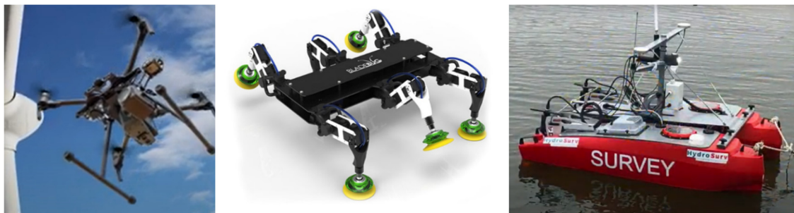
Figure 6. Pictures of an inspection drone under development within the MIMRee project [92], BladeBUG [89], and an unmanned surface vehicle (USV) for autonomous survey operations [94]. Courtesies of MIMRee, BladeBUG and HydroSurv respectively.
