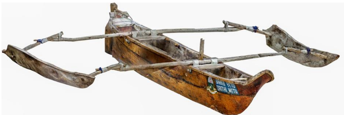
Fig. 2—Screen grab of a 3D digital model of the Bahari Yetu, Urithi Wetu , the extended dugout ngalawa built in 2019 by Mzee Alalae Mohamed. (Image: Authors & Alessandro Ghidoni)
