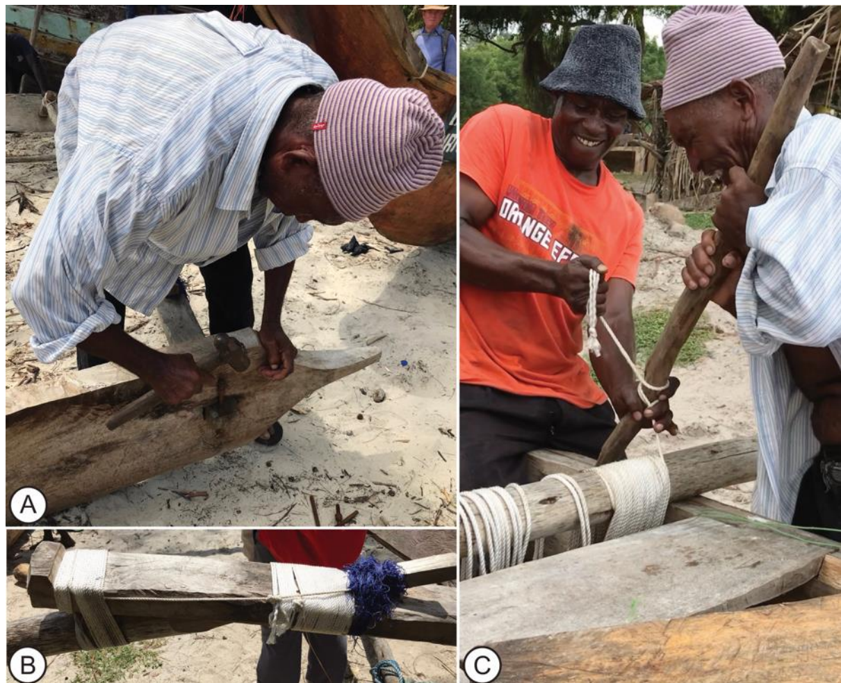
Fig. 22—Outrigger jointing and lashing: (A) the through-teazle-tenon jointing of the outrigger float to the outrigger stanchion; (B) the through-mortise jointing and lashing of the outrigger stanchion to the outrigger boom; (C) Alalae and his assistant lash the boom to the dedicated beam fixed within the hull (Images: Lucy Blue)
