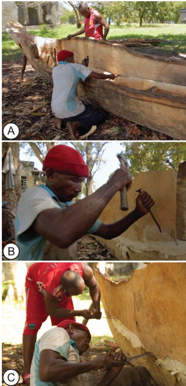
Fig. 21—(A) Marking out sections of the extension plank edge to be removed, using the boatbuilder's pen; (B) temporary nails hold the plank in place during shaping; (C) cutting along the seam with a pruning saw to achieve a tight seam. (Images: Elgidius Ichumbaki and Tobias Minzi)
