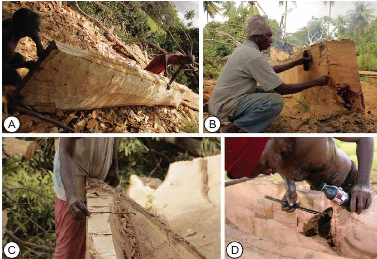
Fig. 6—Measuring and marking implements used on the ngalawa build: (A) string and small nails to anchor it, sometimes used with home-made ink; (B) straight sticks used to evaluate symmetry; two types of pen ( kalamu )—(C) a simple stick dipped in ink to mark out cut lines, and (D) a forked stick with adjustable spacer, used with ink. (Images: Elgidius Ichumbaki and Tobias Minzi)
