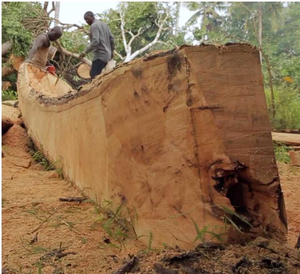
Fig. 13—The state of the hull after almost all reduction using the chainsaw has ended. Only the rake of the stern—marked by the line—has yet to be cut. (Image: Tobias Minzi)
