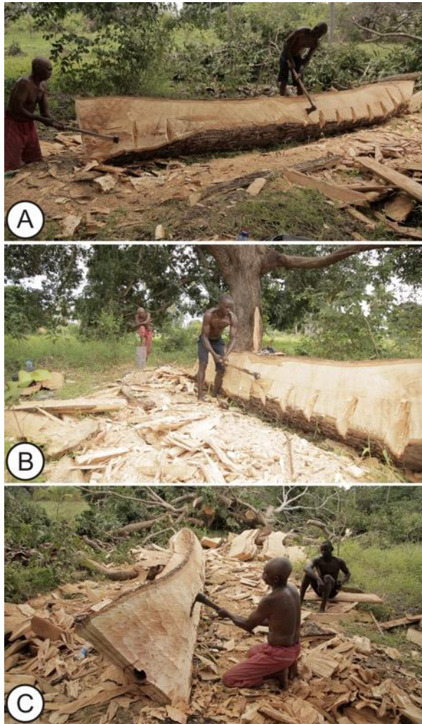
Fig. 17—Reducing the exterior of the dugout: (A) cutting vertical incisions using a felling axe; (B) removing material between the vertical incisions; (C) fairing the hull surface using a foot adze. (Images: Tobias Minzi)
