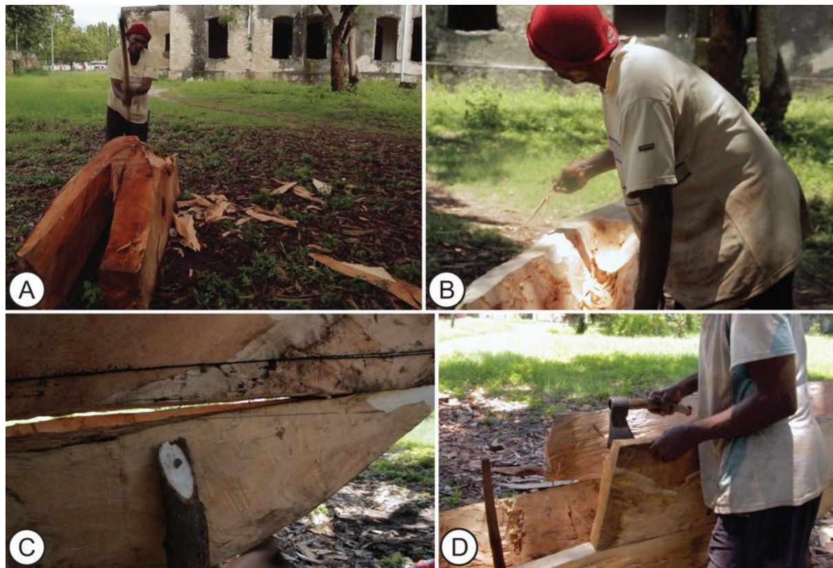
Fig. 20—(A) Alalae roughly shapes the kasama prow timber with a felling axe; (B) marking excess material for removal using the forked pen ( kalamu ); (C) parallel lines marked on the kasama and the bow determine the material, mainly on the former, that will be reduced; (D) the butt joint of the kasama to which the extension plank will be joined. (Images: Elgidius Ichumbaki and Tobias Minzi)
