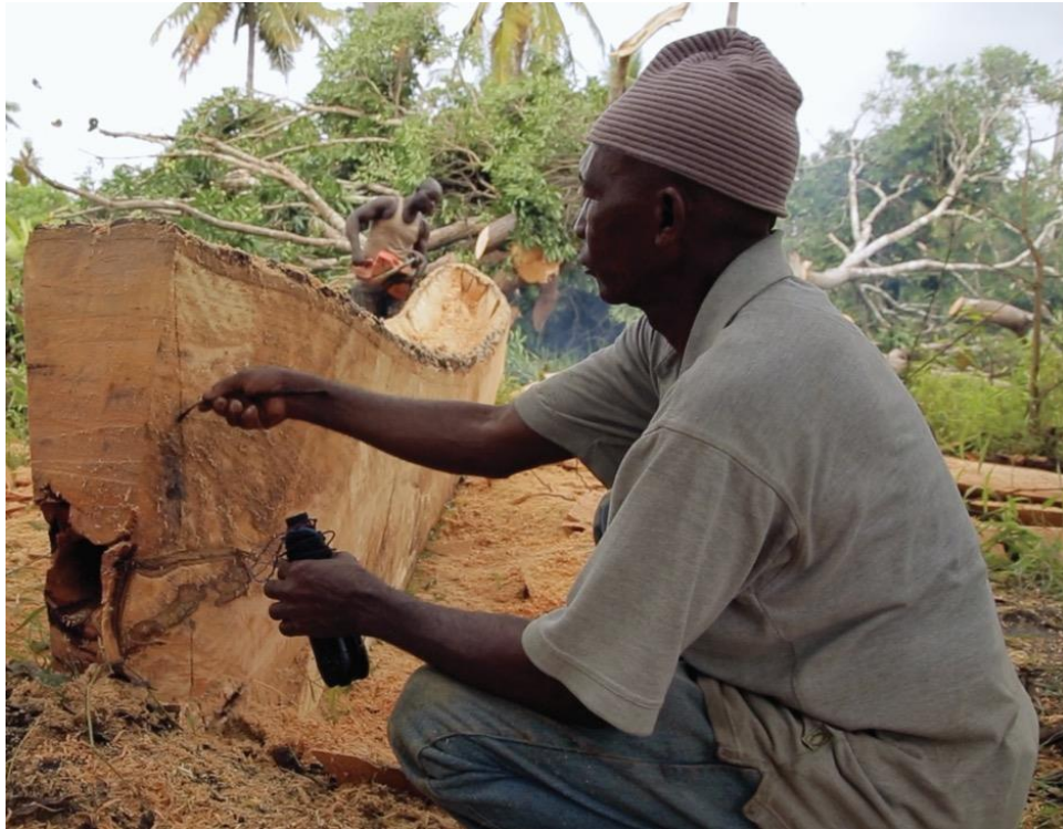
Fig. 12—Alalae marks out the intended rake of the stern. (Image: Tobias Minzi)
