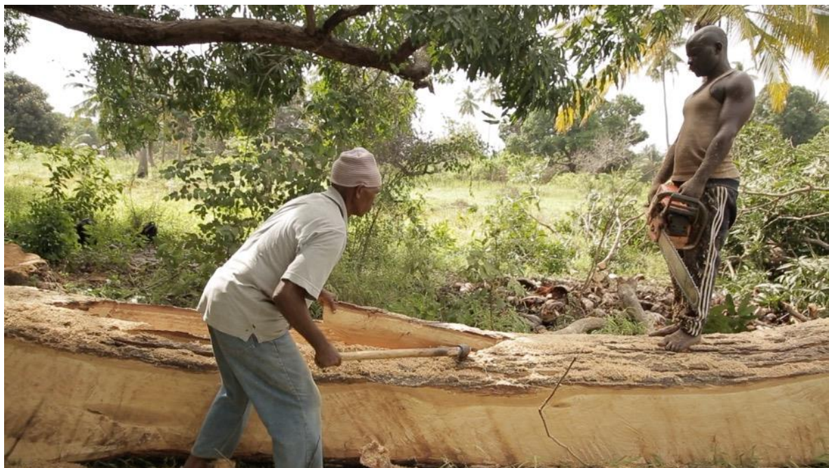
Fig. 10—Removing segments of log that were cut using the chainsaw. (Image: Tobias Minzi).
