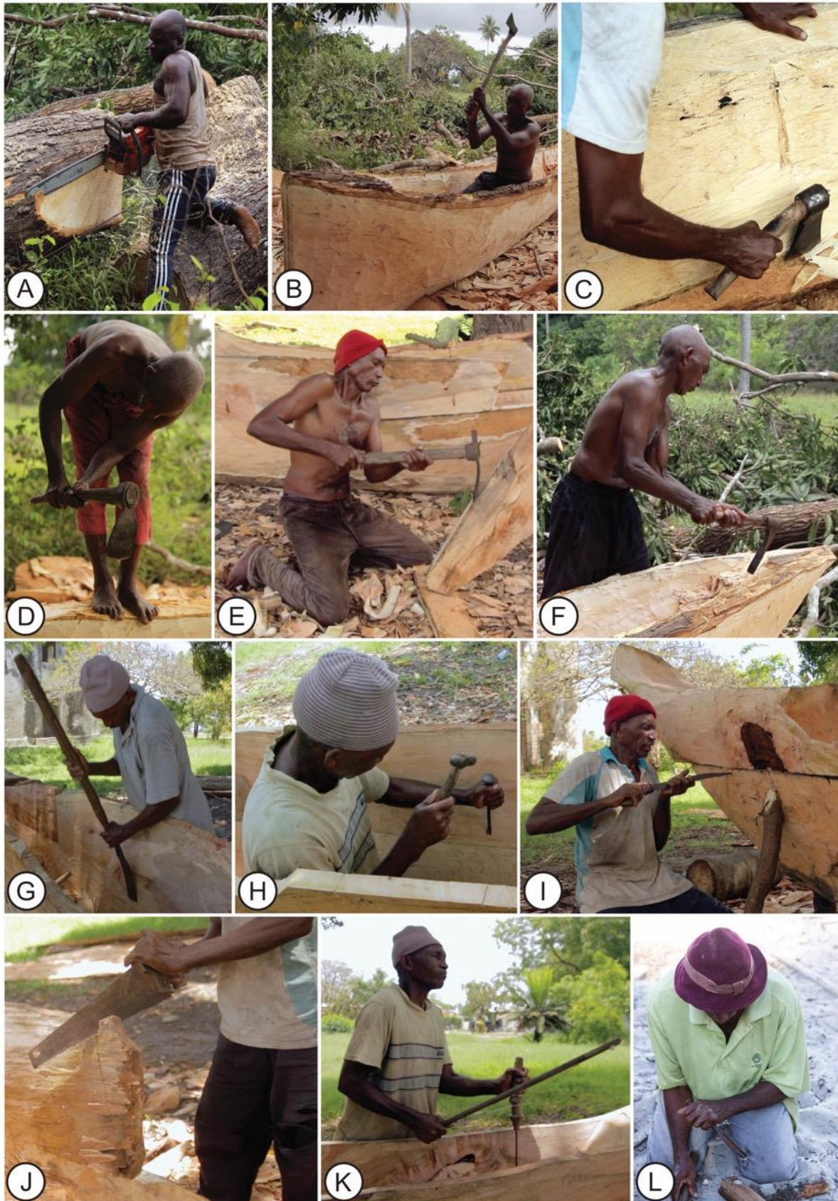
Fig. 5—Tools used on the ngalawa build: (A) Chainsaw; (B) Felling axe; (C) Hand axe with offset handle; (D) foot adze; (E) shipwright's adze; (F) hand adze with narrow blade; (G) ship's slice; (H) flat chisel; (I) pruning saws; (J) hand saw; (K) bow drill; (L) straight gouge, (Images: Elgidius Ichumbaki and Tobias Minzi).
