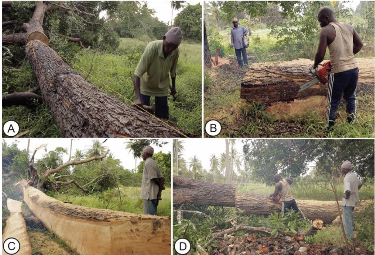
Fig. 9—Rough-shaping the dugout with a chainsaw: (A) Alalae marks out the line of the ‘proto-sheer’ with a hand axe; (B) tapering the stern; (C) shaping the forward end of the dugout to receive (ultimately) the kasama prow timber; (D) reducing the sides outside the marked proto-sheer line. (Images: Elgidius Ichumbaki and Tobias Minzi)
