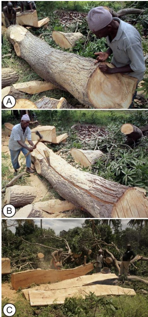
Fig. 11—Cutting the planks: (A) marking out by flicking a line of inked string; (B) splitting off the through-and-through-cut planks with a wedge. (Images: Tobias Minzi).
