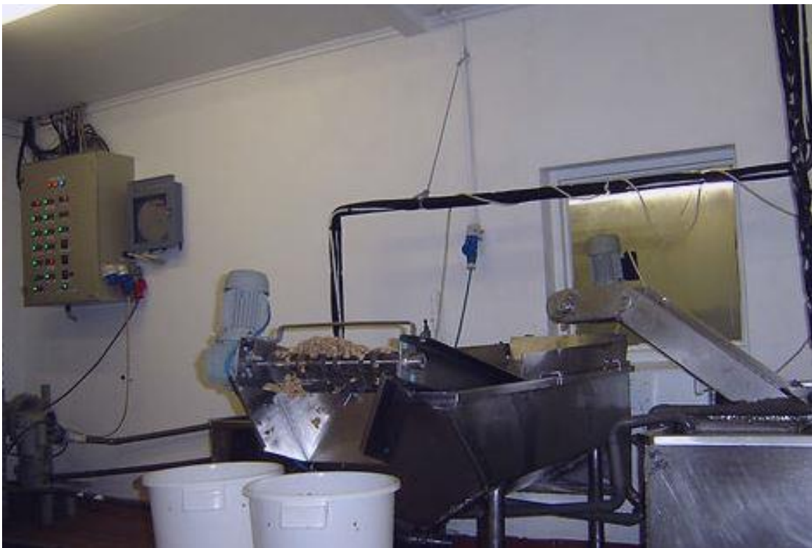
Photograph 18. Computer-controlled cockle cooking and cooling
