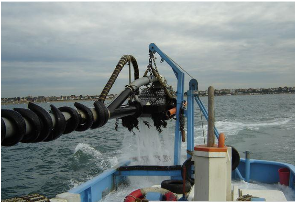
Photograph 3. Sophie Jayne flushing her dredging gear.
