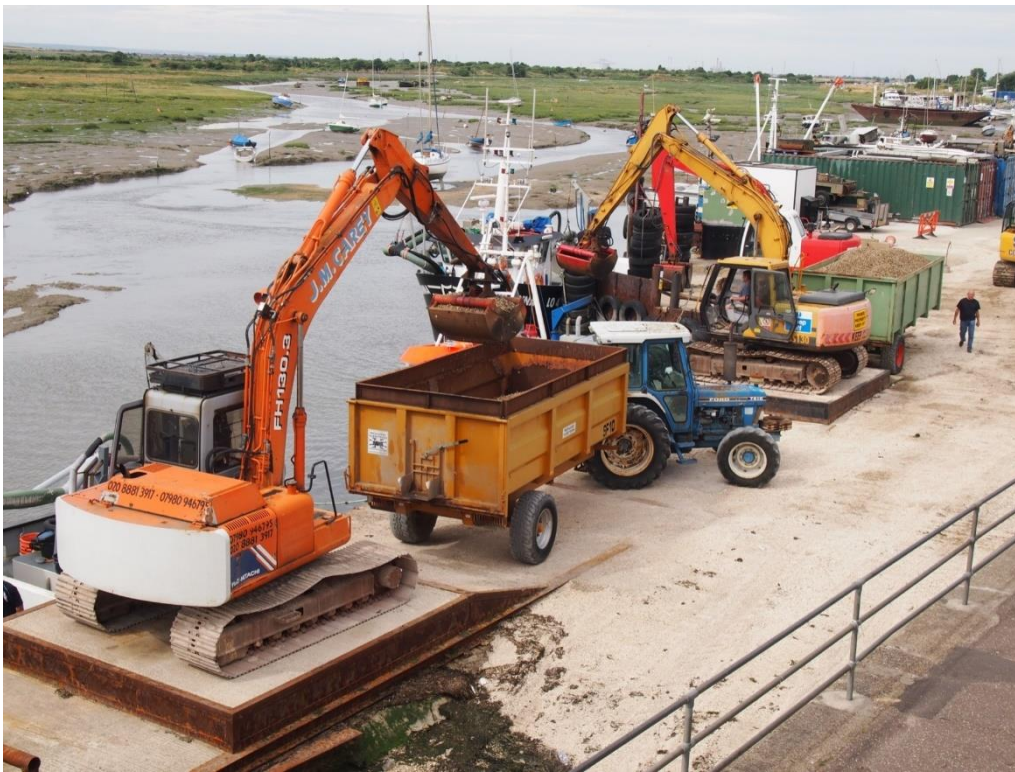
Photograph 7. Hydraulic grab unloading cockle into a tipper trailer
