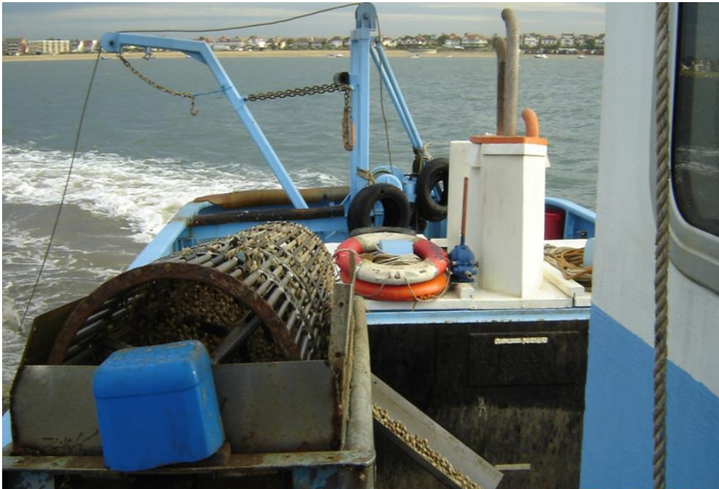
Photograph 2. Hydraulic suction dredge deployed for harvesting
