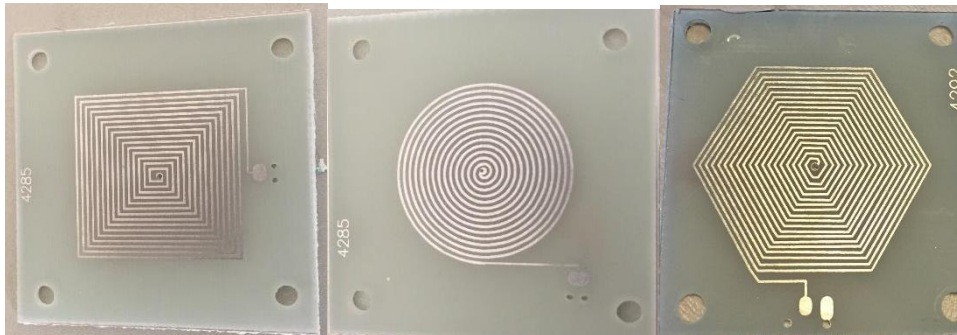
Figure 6.7. (a) Square, (b) Circular, (c) Hexagonal structure for the input and output inductor.
