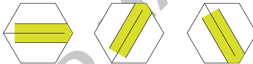
Figure 3: Three possible orientations of a DSLJ damper in a hexagonal cell.
