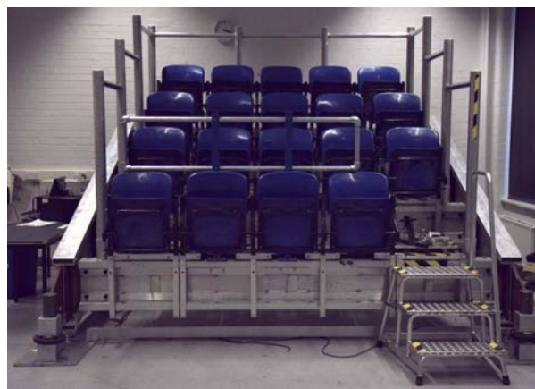
Figure 1: Experimental setup – instrumented grandstand in The University of Sheffield.
