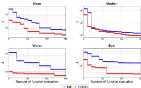
Fig. 9 Convergence of GA based tuning of PID/FOPID controllers.
