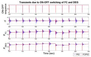
Fig. 12 Transients due to on-off switching of the actuators.
