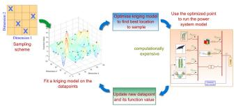
Fig. 3 Schematic of kriging based optimization method.
