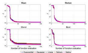
Fig. 7 Convergence of five kriging methods for PID controller.
