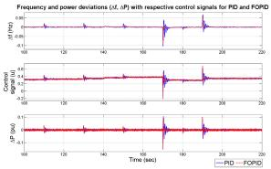
Fig. 5 Frequency deviation, control signal and power deviation of the microgrid with best obtained PID/FOPID controllers.
