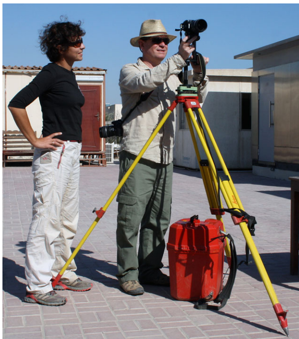
Figure 5. The nodal-ninja arm, holding the Nikon digital SLR camera at the same focal point as that of the Leica HDS6000 laser scanner (Image: A. Wetherelt).
