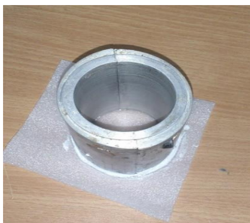
Figure 3. Curing mold used for sample preparation.
