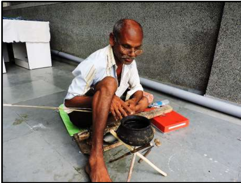
Figure 6.6: A bead-maker drilling a bead using a bow drill that has diamond tips to drill the beads. He drills both polished and unpolished beads, the processes of drilling and polishing are done in either order
