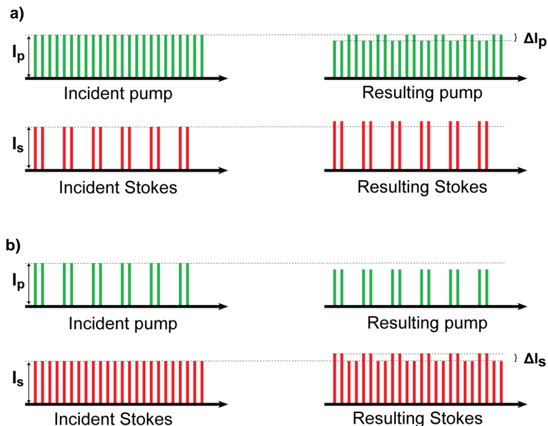
Figure 3.7: The detection mechanism of (a) Stimulated Raman loss (SRL) and (b) Stimulated Raman gain (SRG), adapted from [169].
