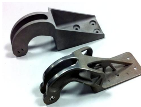
Figure 2.3. Original and optimised engine nacelle hinges for A320 airliners (Tomlin and Meyer 2011).
