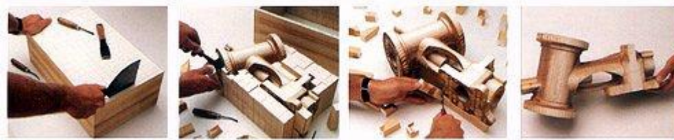
Figure 5.3. Removal of laminated object manufacturing (LOM) support structure (Cubic Technologies, Inc.).
