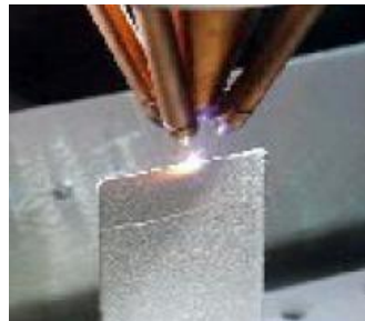
Figure 2.22. Jet nozzle deposition during LENS sintering process (Optomec 2012).
