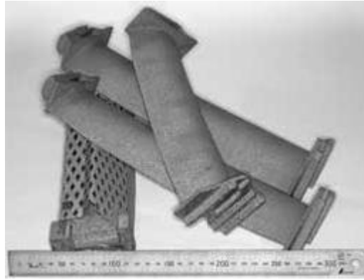
Figure 2.25. Parts manufactured by Electron Beam Melting (Arcam 2012).
