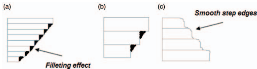
Fig. 3 Filleting effect caused by flow of molten polymer for (a) downwards-oriented facets, (b) the same but inhibited by surface tension to only partially smooth, thick layers. For (c) upward-facing facets, filleting is minimized although surface tension may smooth sharp corners
