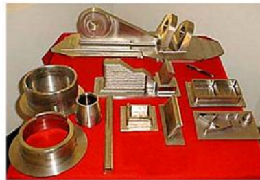
Figure 2.23. Laser engineering net shaping: parts fabricated on Ti alloy (Hedges 2004).
