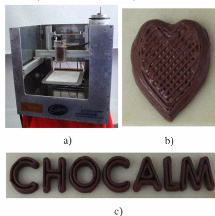
Figure 4. a) ChocALM machine, b) cellular chocolate heart, c) ChocALM logo made by Chocolate.
