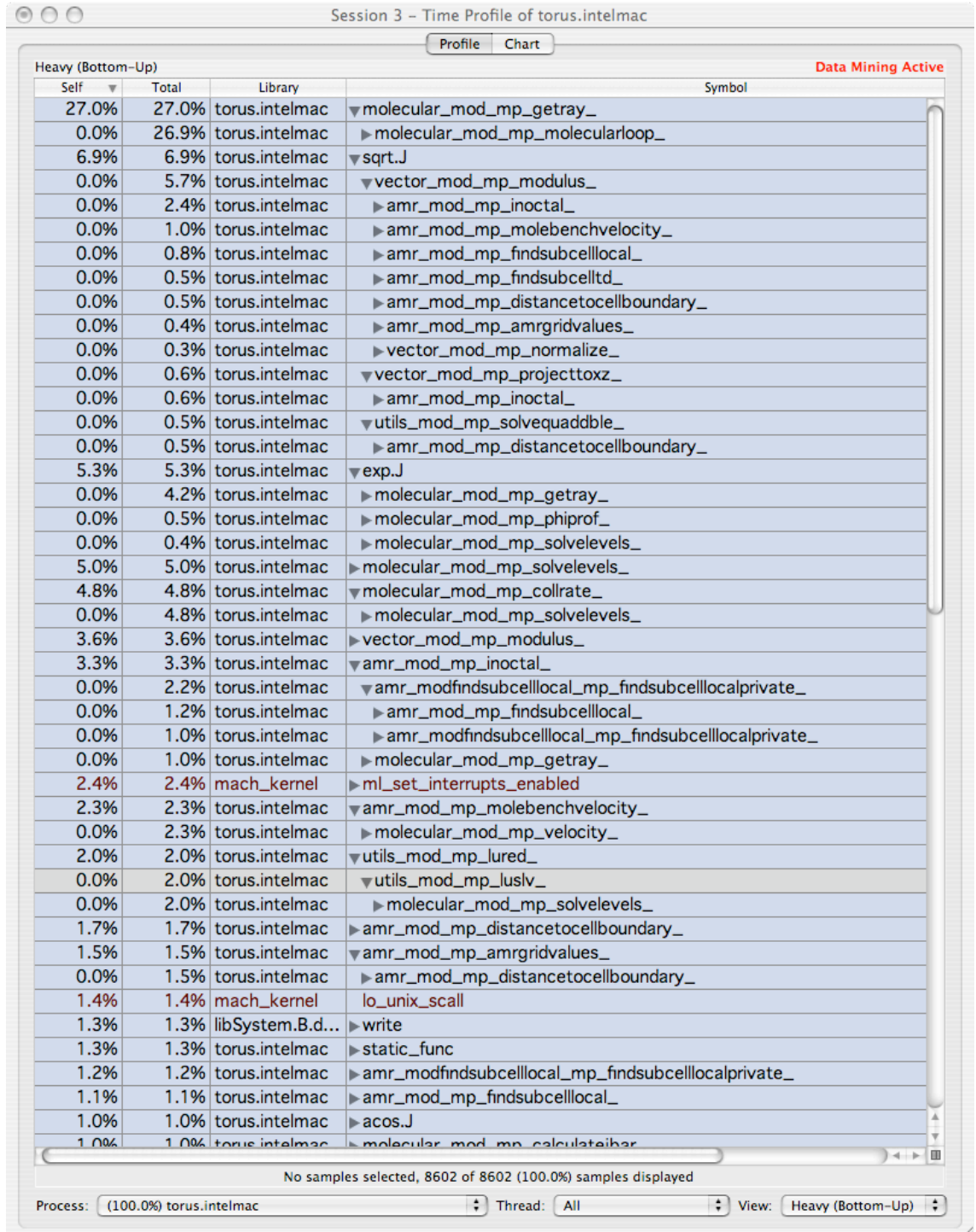
Figure 3.8: This screen capture of Shark profiling tool output at subroutine level shows the time spent in each subroutine during a sample of 30 seconds from the fixed ray stage.
