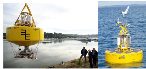
Figure 2: South Western Mooring Test Facility (SWMTF) buoy; launch operation (left); in operation on site (right)
