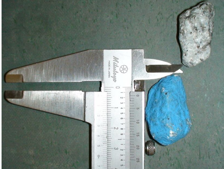
Plate 4.3: A picture of coarse particles placed before a test (measured using a mitutoyo vernier calliper)
