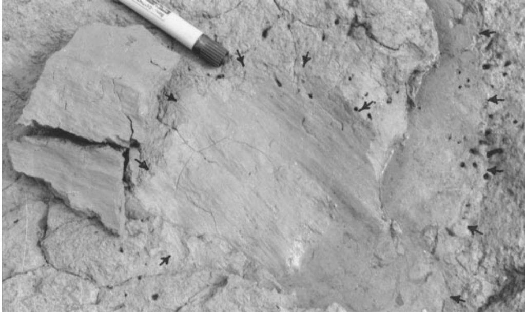
Fig. 13. Slickensided failure surface (arrowed), Eastern Palaeochannel. Spirit marker for scale
