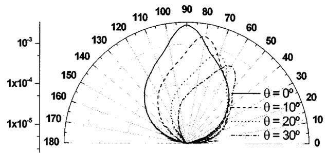
FIG. 3. Experimental angle dependent transmission spectrum of the structure having concentric rings on both surfaces, at the resonant frequency of the sample for incident angles of  $0^\circ$ ,  $10^\circ$ ,  $20^\circ$ , and  $30^\circ$ . (Note for non-normal incidence the exit face of the plate is rotated by the incidence angle relative to the direction of the incident beam which defines  $-90^\circ$  in this figure.)
