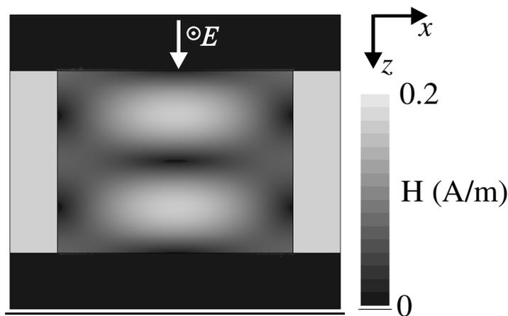
**Figure 4.** Time-averaged magnetic field magnitude within a slit of  $l = 25$  mm,  $w = 80 \mu\text{m}$  and  $t = 19.58$  mm. Resonant mode  $N = 2$ ,  $M = 1$  is shown. Incident microwave beam and coordinate axes are shown, corresponding to the computer model. Incident electric field magnitude =  $0.0027 \text{ A m}^{-1}$ .
