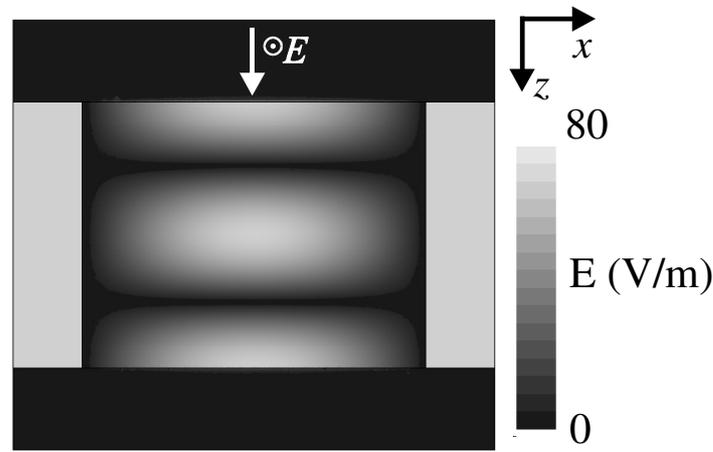
**Figure 3.** Time-averaged electric field magnitude within slit  $l = 25$  mm,  $w = 80 \mu\text{m}$  and  $t = 19.58$  mm. Resonant mode  $N = 2$ ,  $M = 1$  is shown. Incident microwave beam and coordinate axes are shown, corresponding to computer model. Incident electric field magnitude =  $1 \text{ V m}^{-1}$ .
