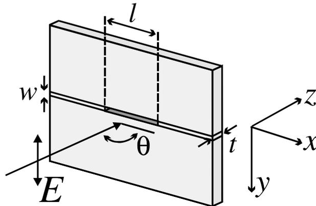
**Figure 1.** Experimental setup with dimensions, microwave polarization and axes labelled. Axes chosen to correspond to the computer model.
