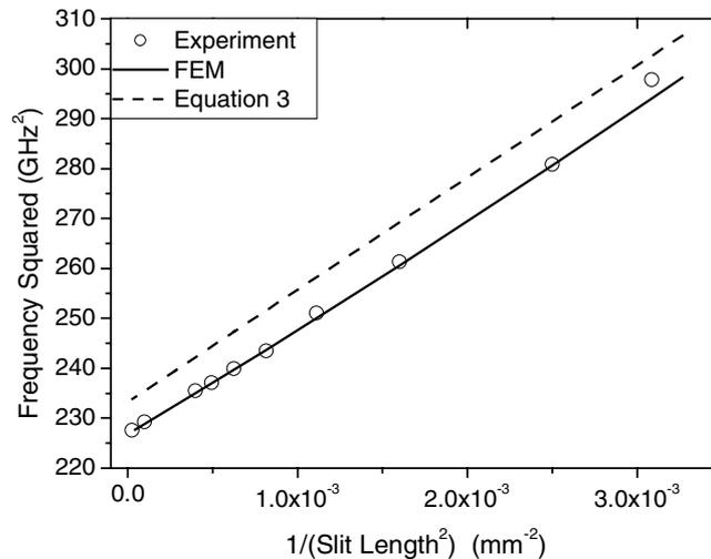
**Figure 2.** Experimental data, square of resonant frequency against square of inverse slit length,  $18 < l < 200$  mm for a slit width,  $w = 80 \mu\text{m}$  ( $\circ$ ). FEM prediction (—) and equation (3) prediction (----).
