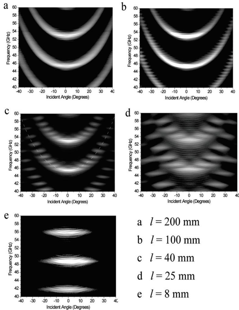
**Figure 5.** Experimental data showing resonant transmission of a finite length single slit as a function of slit length. Transmission intensity of slit lengths (a) 200 mm, (b) 100 mm, (c) 50 mm, (d) 40 mm and (e) 8 mm shown are plotted over frequency range  $40 < f < 60$  GHz and angle range  $-40 < \theta < +40^\circ$ . Light areas indicate strong transmission.
