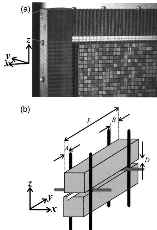
FIG. 1. (a) Photograph of a section of the sample used in this study. The length and width of each rod in the array are approximately 36 and 4 mm, respectively, and the size of the complete sample has side lengths of around 385 mm. (b) Schematic diagram illustrating the geometry of the fiber (black and dark gray) with respect to the metal rods. The white area (that extends along the entire length of the rod) indicates the region over which the fields illustrated in Fig. 3 are calculated.
