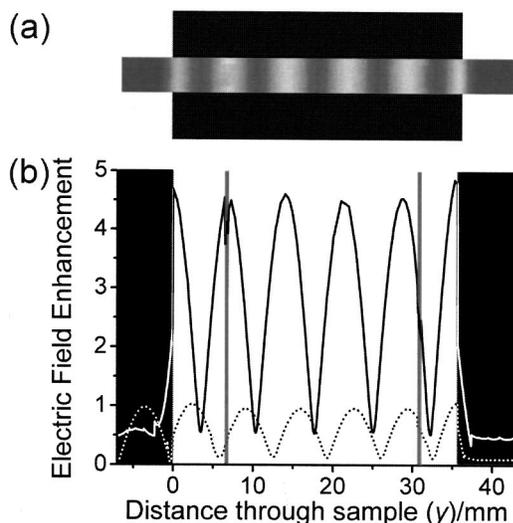
FIG. 3. (a) Calculated electric field intensity in the vicinity of the cavity and in the plane described in Fig. 1(b) on resonance of the 20.3 GHz mode. (b) Line graph showing the on (20.3 GHz) and off resonance (22.0 GHz) electric field enhancement along the center of the cavity (solid and broken lines, respectively). The field enhancement outside the sample is shown in the black regions, and the positions of the line are also illustrated (gray lines).
