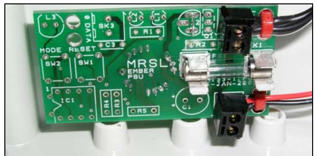
Figure 5: PCB for 'sparse' version without any microprocessor components. Note wire link across Q2 and cable ties securing flying leads. Also note the three mounting bushes below the PCB – hole in case must be drilled in the appropriate side of the case.
