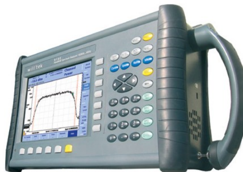
Figure 3.12: Willtek 9102 Hand-held Spectrum Analyser
