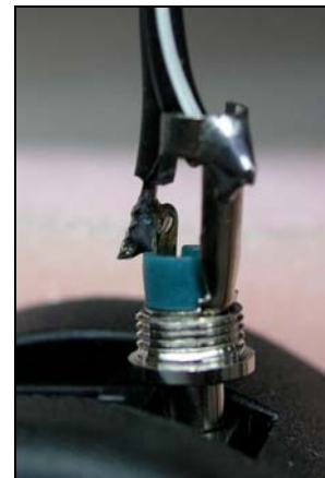
Figure 4: soldering of bell wire to 1.3mm power plug. Note absence of plug housing – no room in case.
