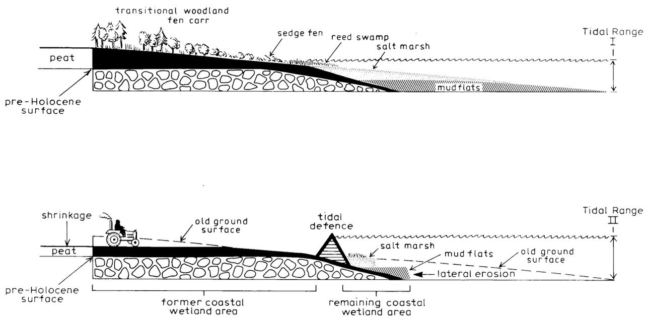
Figure 6.2 Schematic representation of the effects of coastal squeeze.
