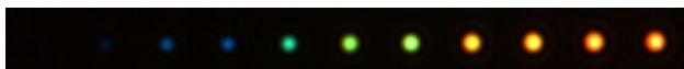
Figure 1.1.1: A dark-field microscope image of 50nm thick silver discs (diameter 50 to 150nm) surrounded by glass. This demonstrates the dependence of the resonance wavelength on the geometry of the particles.
