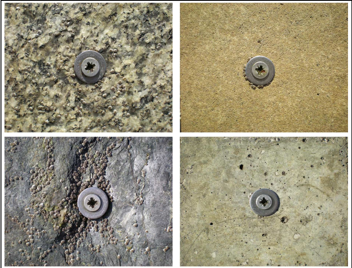
Figure 5-13 Representative photographs of each treatment (Plot PB) at the end of the first year of settlement, November 2008 (clockwise: flame-textured granite, sawn limestone, plain-cast concrete and cleared [slate] platform; washer diameter = 2 cm for scale).
