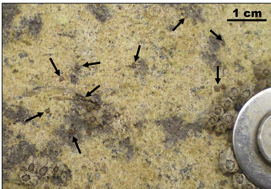
Figure 7-17 Association between weathering of limestone and barnacle recruitment (juvenile recruitment in weathering pits developed after exposure for 14 months at MTL indicated).
