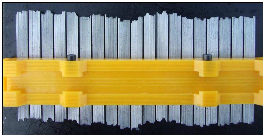
Figure 4-1 Carpenters profile gauge used to assess surface roughness in geomorphology (each pin = 0.8 mm).
