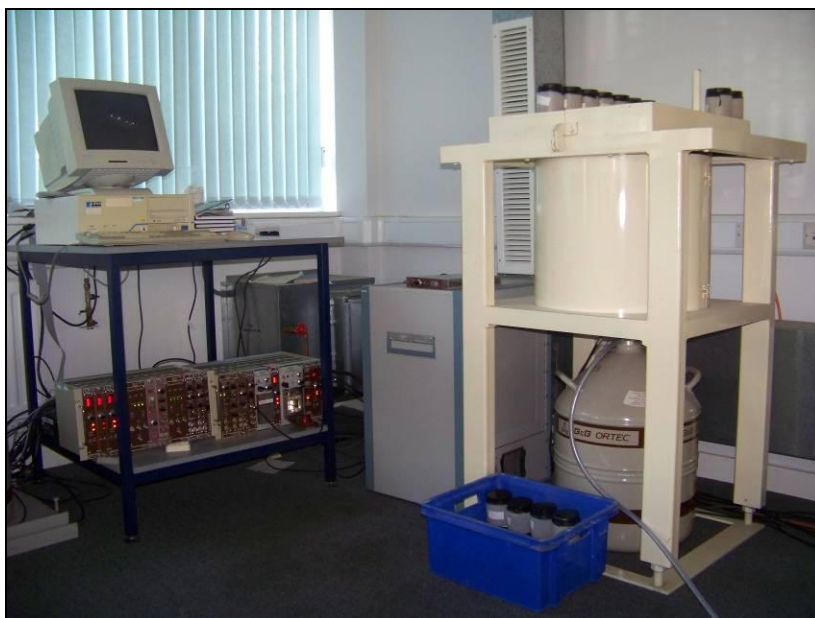
Figure 2.12 ORTEC LO-AX Hyperpure Ge co-axial \gamma -detector (EG&G ORTEC LO-AX HPGe), coupled to a multi-channel analyser and computer control device
