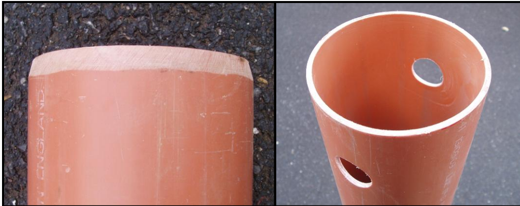
Figure 2.6 Details of the prepared plastic coring tube
