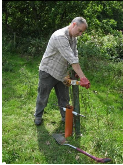
Figure 2.8 Floodplain core extraction
