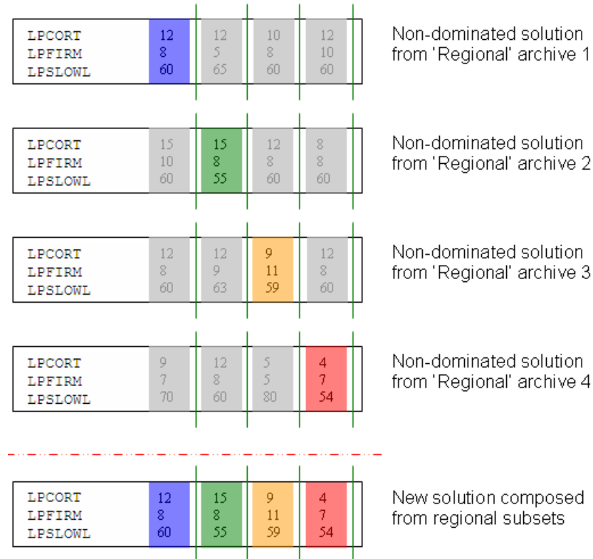
Figure 4.1: Region ‘splicing’. Parametrisations are maintained in separate archives each concerned with evaluating dominance for a particular regional parameter subset and the associated TP and FP rates resulting in that region. For evaluation purposes non-dominated parameter subsets are selected from each regional archive and combined to create a new parametrisation that can be evaluated on the STCA system.
