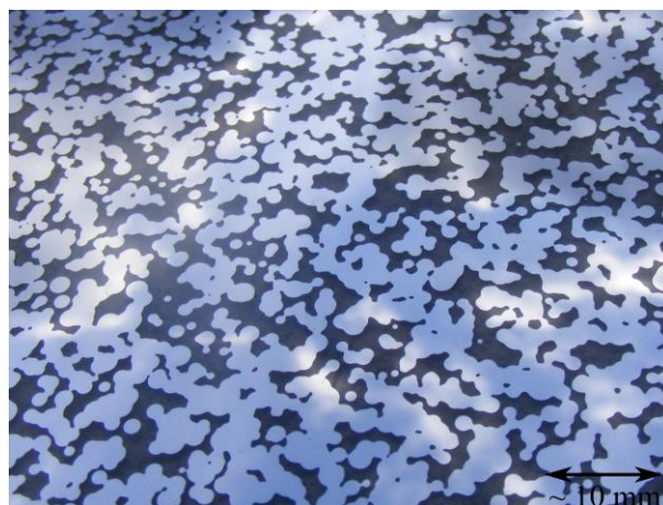
Figure 4.3.4. Image of a random array fabricated from aluminised Mylar ® .
