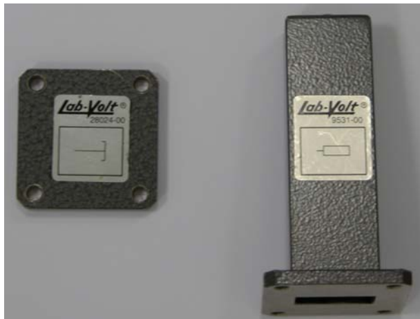
Figure 5-3: Standard loads; a metallic sheet (left) and a matched load (right).
