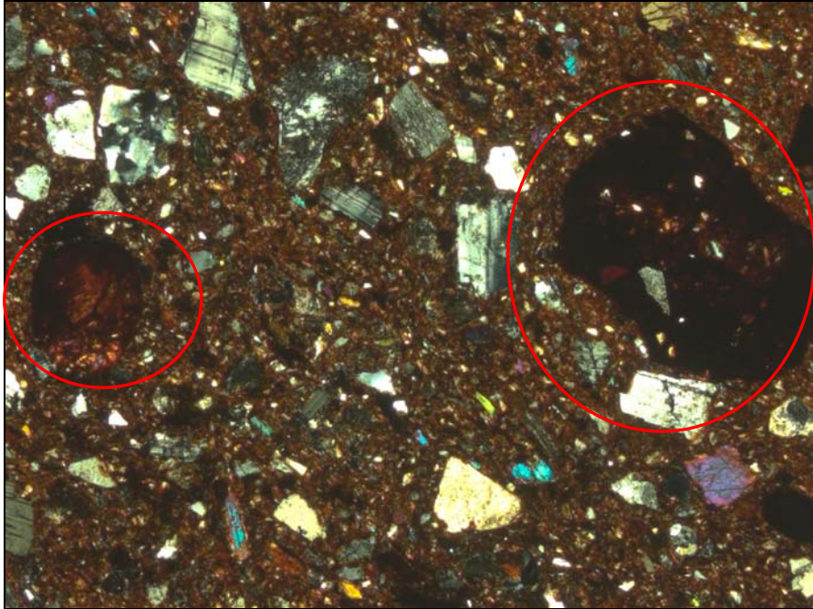
Figure 7:23 Example of well-rounded clay pellets Slide 21 Carngoon Bank (Author's Photomicrograph).
