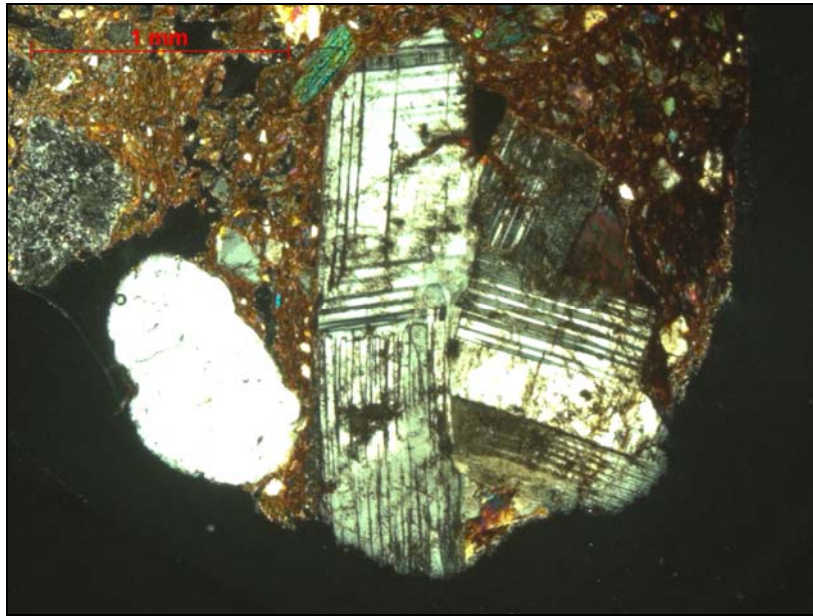
Figure 7:37 Example of Chunky Fabric group with rock fragment containing plagioclase feldspar and quartz, with a well-rounded quartz grain (sand) to the left and greenish blue lath of biotite mica top centre; Slide 74 Winnianton (Author's Photomicrograph).
