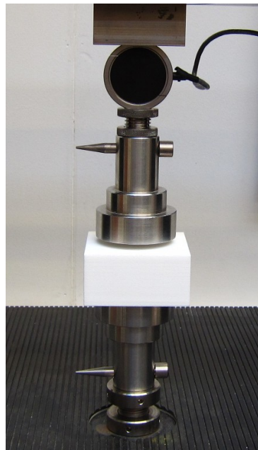
Figure D.1: Loading of the box component. Not visible is a small metal disk 15 mm in diameter on top of the component.
