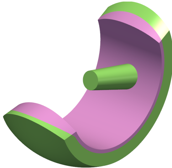
(a) Condylar implant CAD model. The inner (pink) part is used to define the space the lattice structure will occupy.
