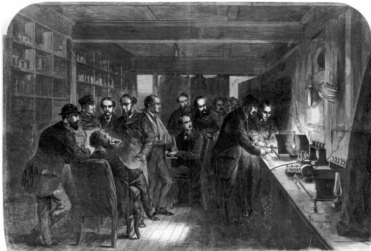
Figure 1. The Great Eastern cable-testing room during the 1866 Atlantic cable expedition. On the right, electricians judge the strength of signals through the cable using the movements of a light beam reflected from William Thomson's 1858 mirror-galvanometer. Illustrated London News , 13 October 1866, 357. Reproduced by permission of the British Library.
