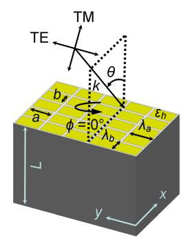
FIG. 1. (Color online) Experimental sample. The holes are of depth L = 30 mm and side lengths a = 8 mm and b = 5 mm. The pitches in the *y*-and *x*-directions are  $\lambda_a = 9 \text{ mm}$  and  $\lambda_b = 6 \text{ mm}$ , respectively. The holes are filled with dielectric (wax),  $\varepsilon_h = 2.25$ . Plane of incidence is shown.
