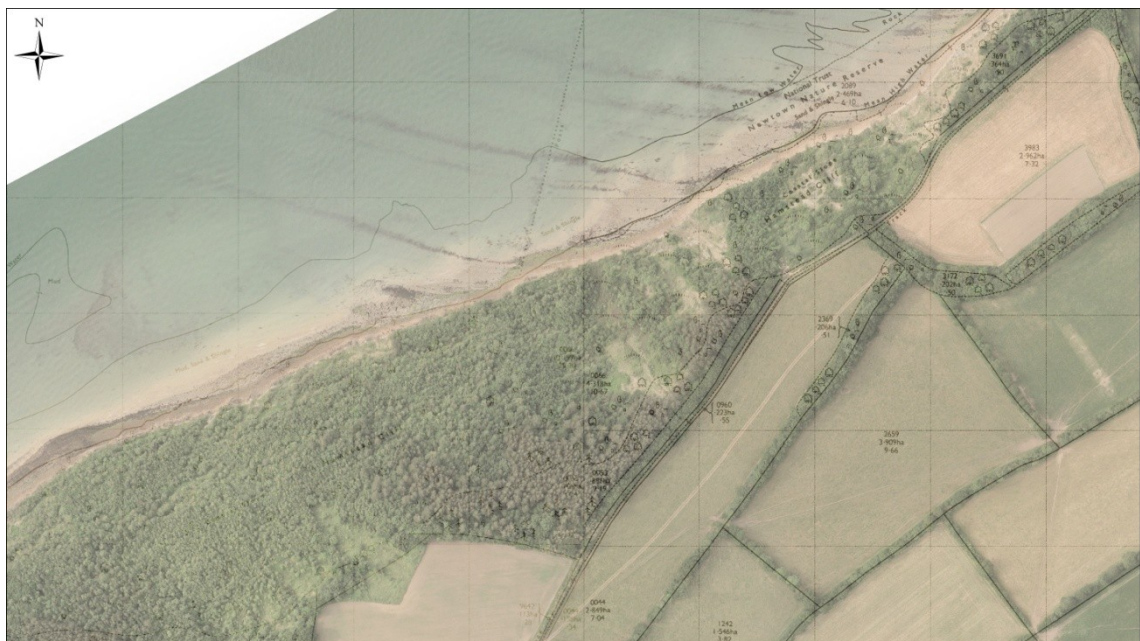
Figure 7.20 Hamstead, west of the Newtown Estuary, illustrating the difficulties of identifying the top of the coastal slope on a wooden and eroding coast. 1975 Ordnance Survey map overlain on 2001 aerial photograph (image courtesy of Channel Coastal Observatory)
