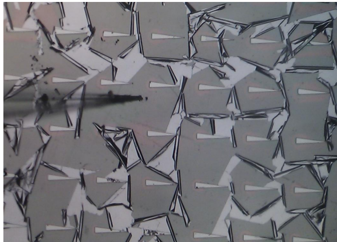
Figure 6.10: Curling of the chromium layer on the photo resist is observed originating at the edges of some triangles. The point of the stretched pipette is also shown.
