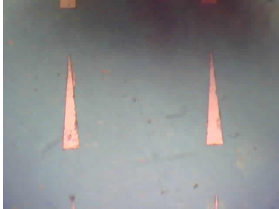
Figure 6.12: Part of a cleaned array of chromium triangles on a PMMA protective layer on an InSb substrate.
