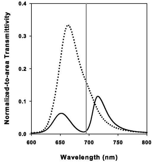
FIG. 3. Normal incidence transmission spectra of a hole array ( $P=380$  nm) covered with undoped PVA (dotted line) and with  $J$ -aggregate doped PVA (solid line). The vertical line at 693 nm indicates the peak of the  $J$ -aggregate absorption band.
