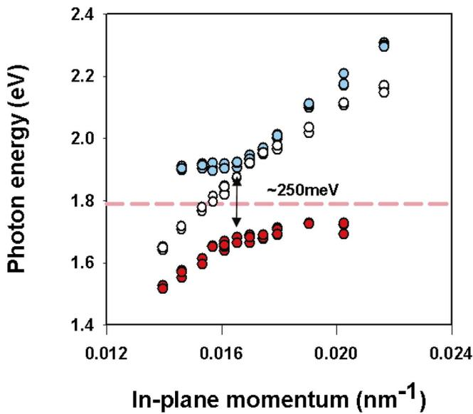
FIG. 4. (Color) Energy dispersion curves for undoped samples (white) and *J*-aggregate doped samples (red and blue) determined by varying the period of the hole arrays. The blue and red dots correspond to the two peaks shown in Fig. 3 with an extended range of period (from 290 to 450 nm), and the red dashed line to the exciton absorption energy.
