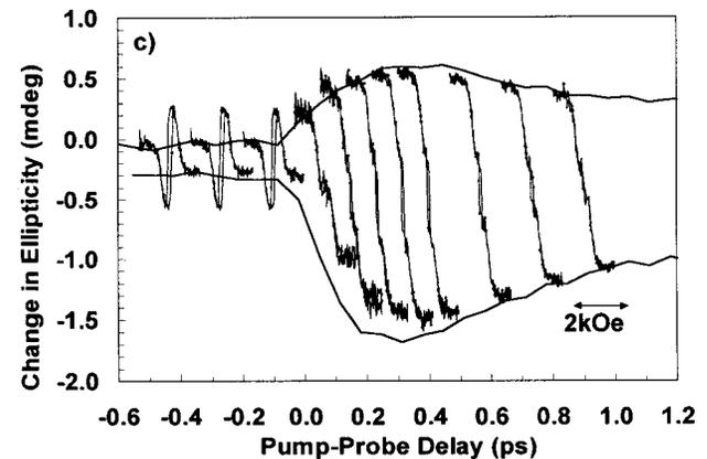
FIG. 3. The time and field dependence of the change in (a) the rotation, and (b) the ellipticity signals is shown. The diamonds show the raw time-resolved measurements at static fields of  $\pm 860$  Oe. The open circles represent half the difference of the signals measured at positive and negative field. The inset in (b) shows the ellipticity signal on a longer time scale. (c) shows field-dependent dynamic ellipticity loops at different time delays. The field scale is indicated.
