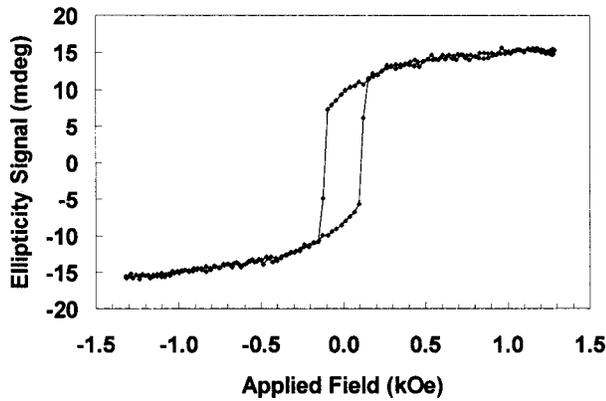
FIG. 2. A static magnetization loop obtained from a measurement of the Kerr ellipticity in the absence of the pump is shown.
