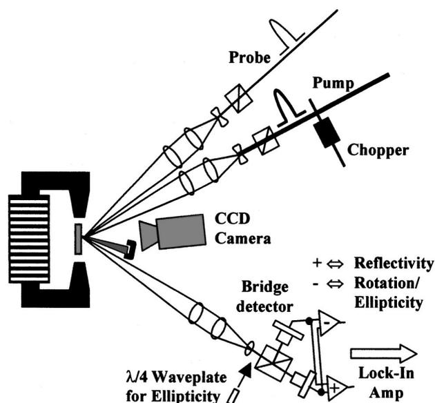
FIG. 1. The measurement configuration used for the pump probe measurements is shown.
