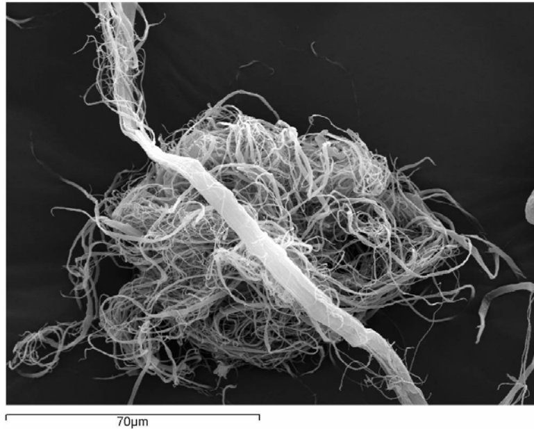
Figure 5.5 Net structure of fine Twaron fibres
