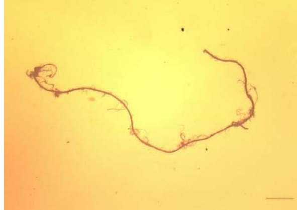
Figure 5.20a Large structural aramid fibre
