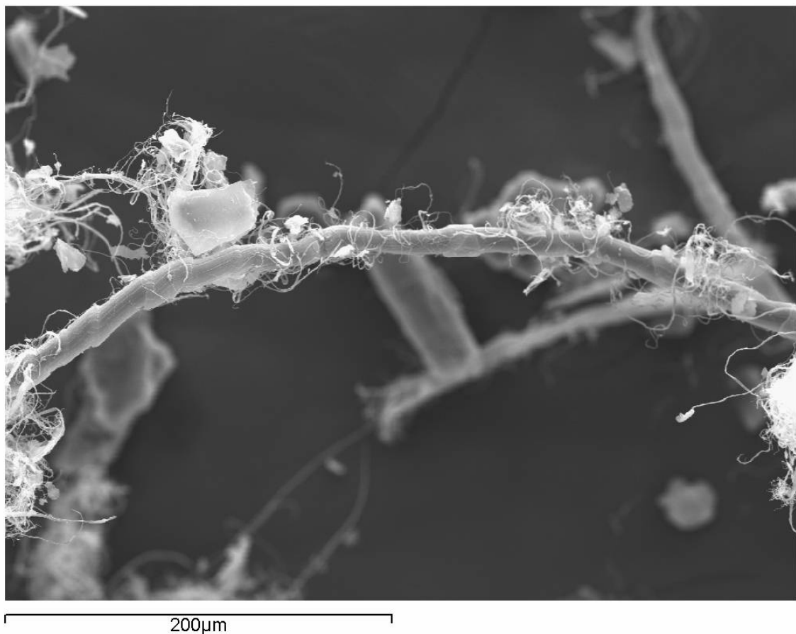
Figure 5.9 Graphite flakes with Twaron hierarchal fibre structure
