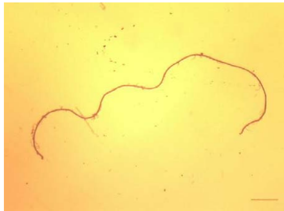
Figure 5.20b Large structural aramid fibre
