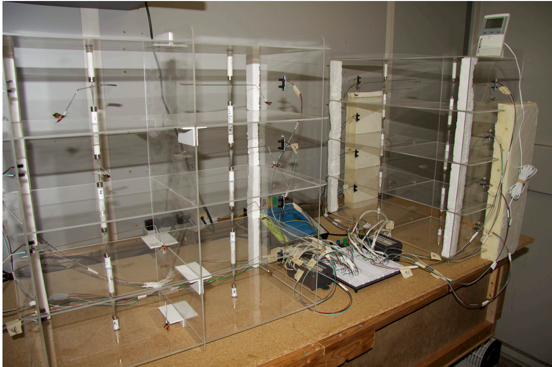
Figure 2. Flight mills structure operating during one of the experimental tests. The second structure on the side mounts two lateral polystyrene supports.
