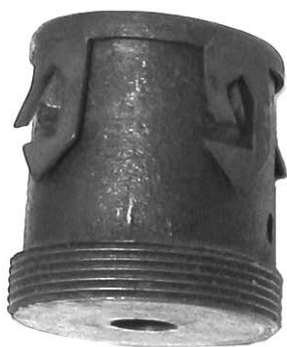
Fig. 48 (right) Cuttaway No. 146 fuze. Note the tape spring which was similar to the tapes used on percussion fuzes for hand and rifle grenades
