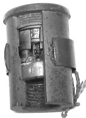
Fig. 49 (left) No. 105B, a simple percussion mechanism
