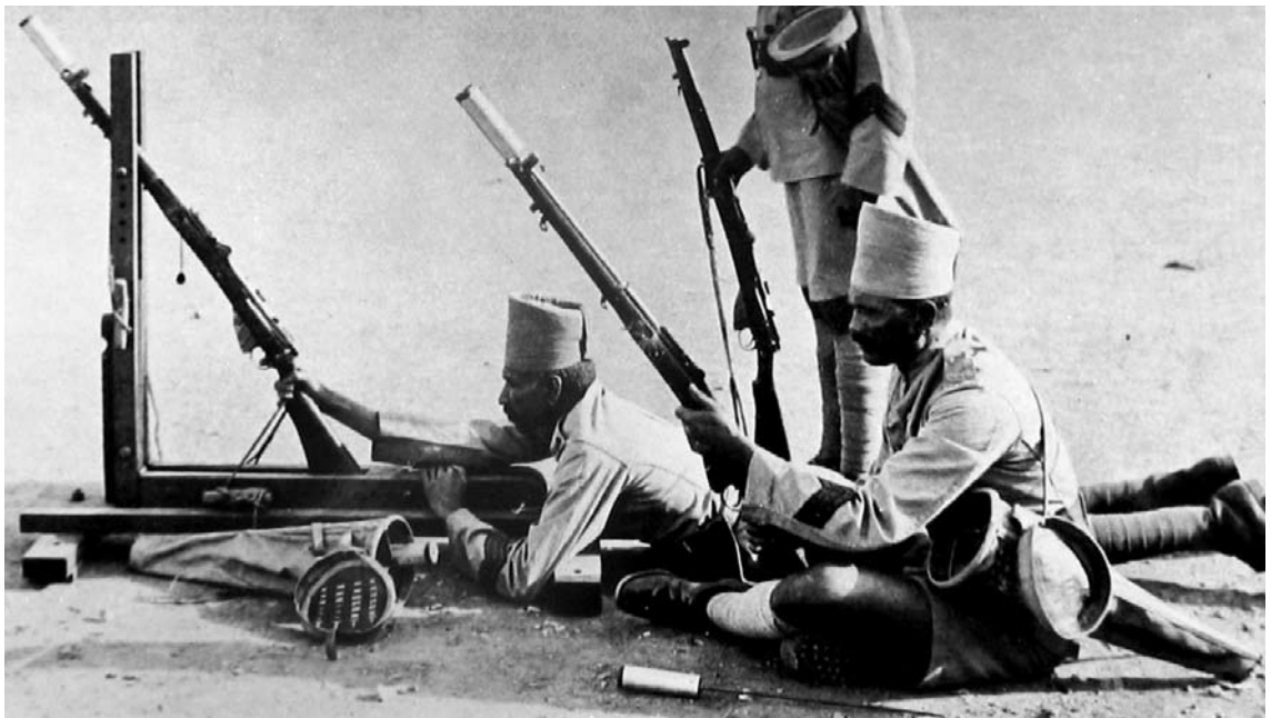
Fig 35 (above) The McClintock rifle grenade, India, 1912. The wooden stand is provided with a butt stop and a movable muzzle rest (pegs in holes) which is positioned according to the aim set by the plumb sight (hanging from the rifle stock). The quiver is for carrying the grenades; its top contains a range table (Royal Engineers Journal)
