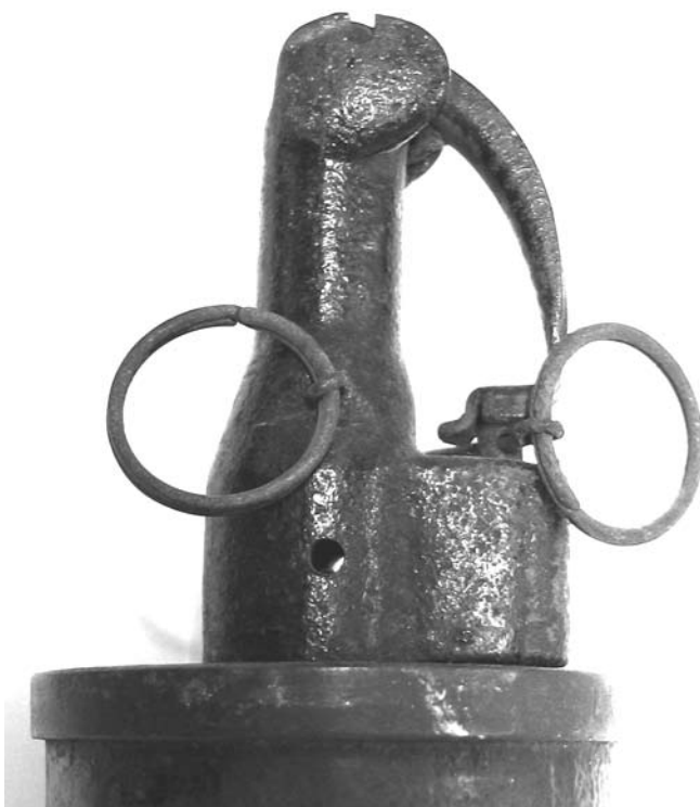
Fig. 43 The time fuze, adapted from the Mills mechanism, used on 3-inch Stokes bombs throughout the war. Note the two safety pins. The left-hand pin prevents the striker from falling, while the right-hand pin prevents a spring-loaded plunger from falling and freeing the lever (author's photograph of example in Norman Bonney's collection)
