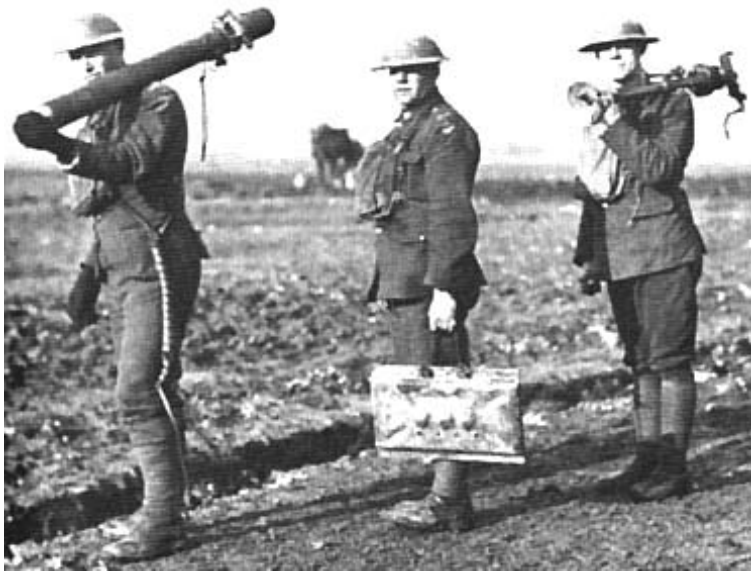
Fig. 74 Part of a Stokes mortar detachment demonstrate the relative ease with which the three elements of the mortar could be carried. The first man carries the barrel, the second the base plate by means of a rope handle, while the third carries the mounting. It is apparent that the men are not over-burdened. This photograph was taken c. 1917
