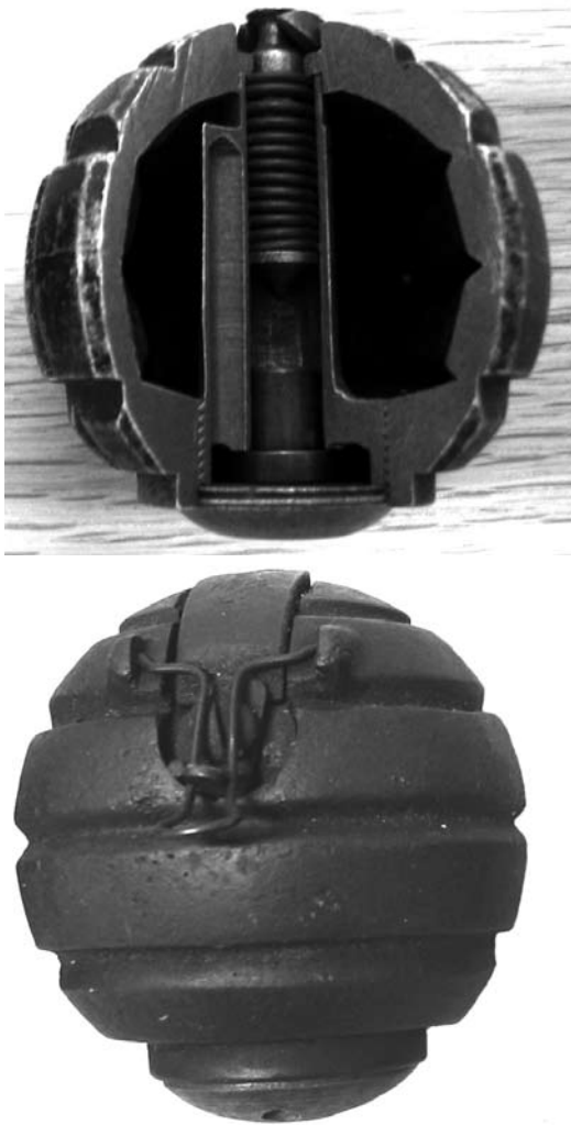
Fig. 25 (left) The Roland hand grenade. The centrepiece, striker and base-plug can be seen clearly in the top photograph, while the lever and safety pin can be seen in the bottom photograph. The forked head of the lever engages the tail of the striker. Note that the grenade is spherical and that the cast body is provided internally and externally with grooves to assist fragmentation. The cutaway is an aluminium demonstration example in which the centrepiece has been cast in one piece for convenience (Author's photographs of specimens in Norman Bonney's collection)
