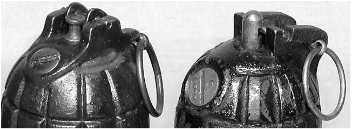
Fig. 28 (above) This illustrates the differences between the No. 5 (left) and No. 36 (right) hand grenades. The tops of the strikers, the flanges which engage the lever trunnions, and the filler holes are all noticeably different. It is clear from this photograph that the notched striker of the No. 36 allows the lever to make a firmer engagement (inert-ord.net)
