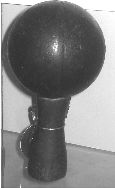
Fig. 1 British improvised hand grenade from the siege of Mafeking, 1899. Note the wooden handle. The grenade is a time-fuzed iron sphere. The metal disk is an identification tag (Norman Bonney)
