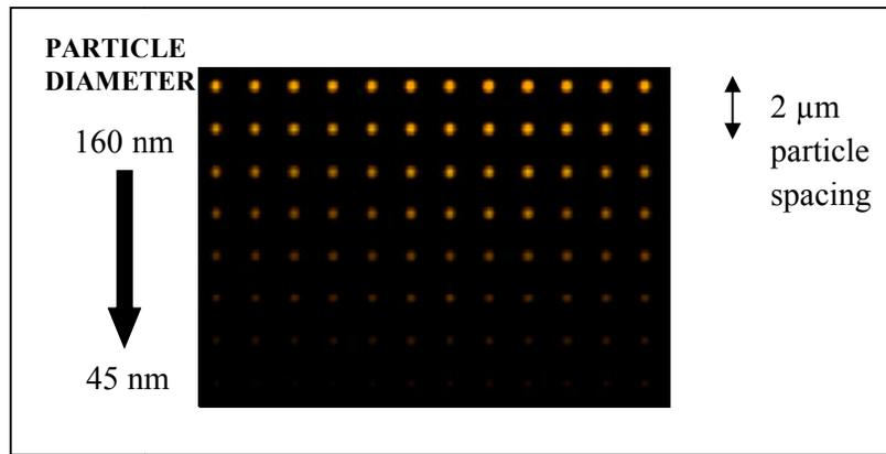
**Figure 4.10:** CCD image obtained from a dark field microscope used to observe scattering from Au discs with height 35 nm and diameters ranging from 45 nm to 160 nm. The image has been normalised to the lamp spectrum.
