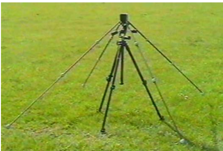
Figure 3.9. An example of the calibration frame used to calculate the DLT parameters
