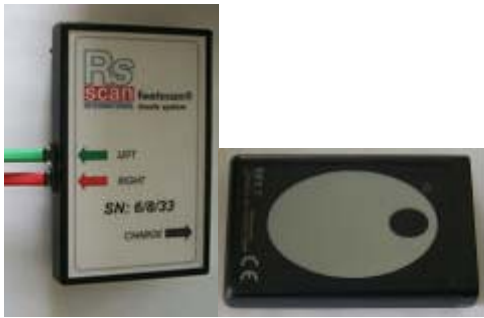
Figure 3.8. An example of the data logger and remote control activator
