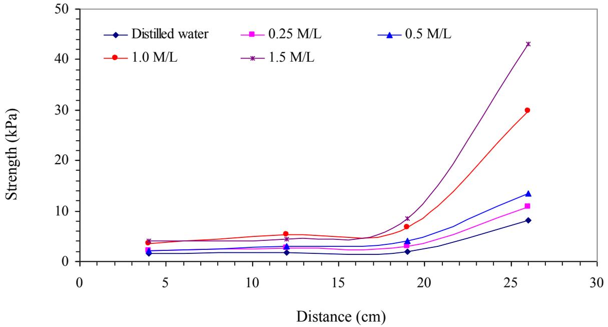
**Fig.9.** Variation of strength along the soil sample
