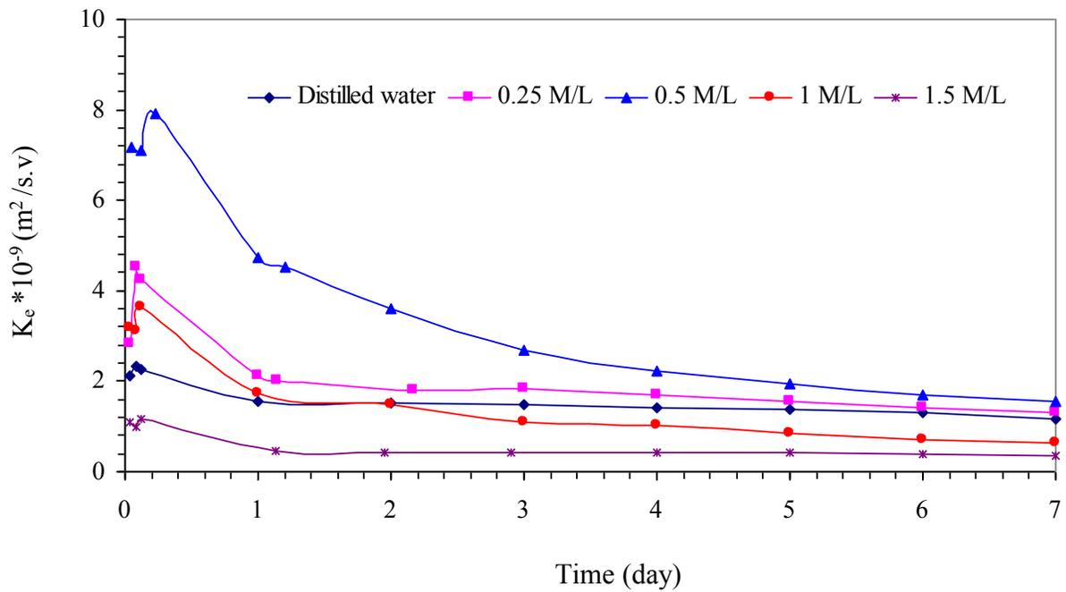
**Fig.6.** Variations of  $K_e$  with time during different tests. DW= Distilled water
