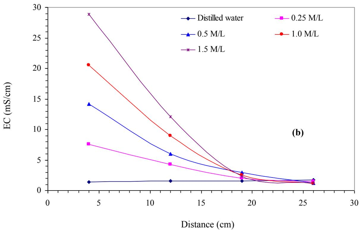
**Fig.10.** Variations of pH (a) and EC (b) along the soil sample
