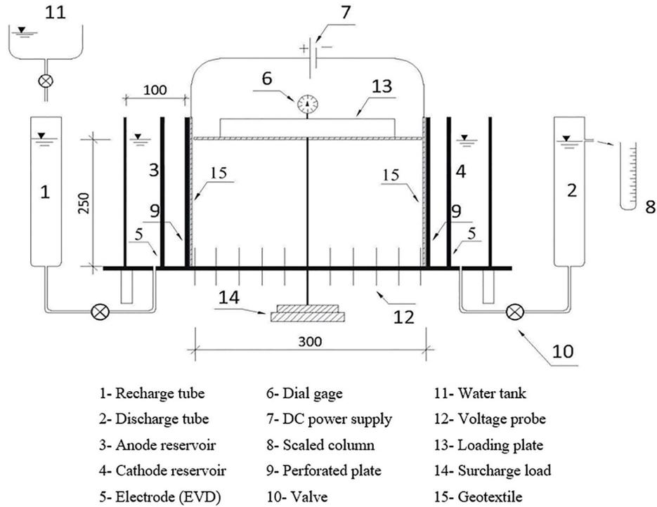
**Fig.2.** Schematic plan of the test set-up (dimensions in mm)
