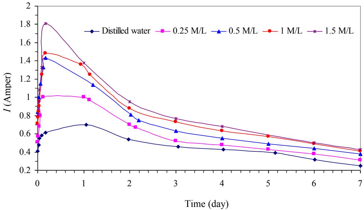
**Fig.7.** Variation of current intensity with time during different tests. DW= Distilled water
