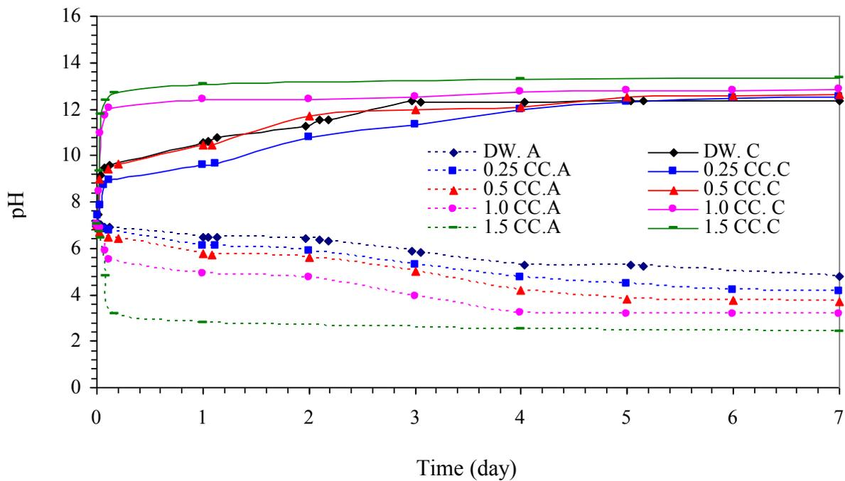
**Fig.3.** Variations of pH with time. DW=Distilled water, CC= Calcium chloride A=Anode, C= Cathode
