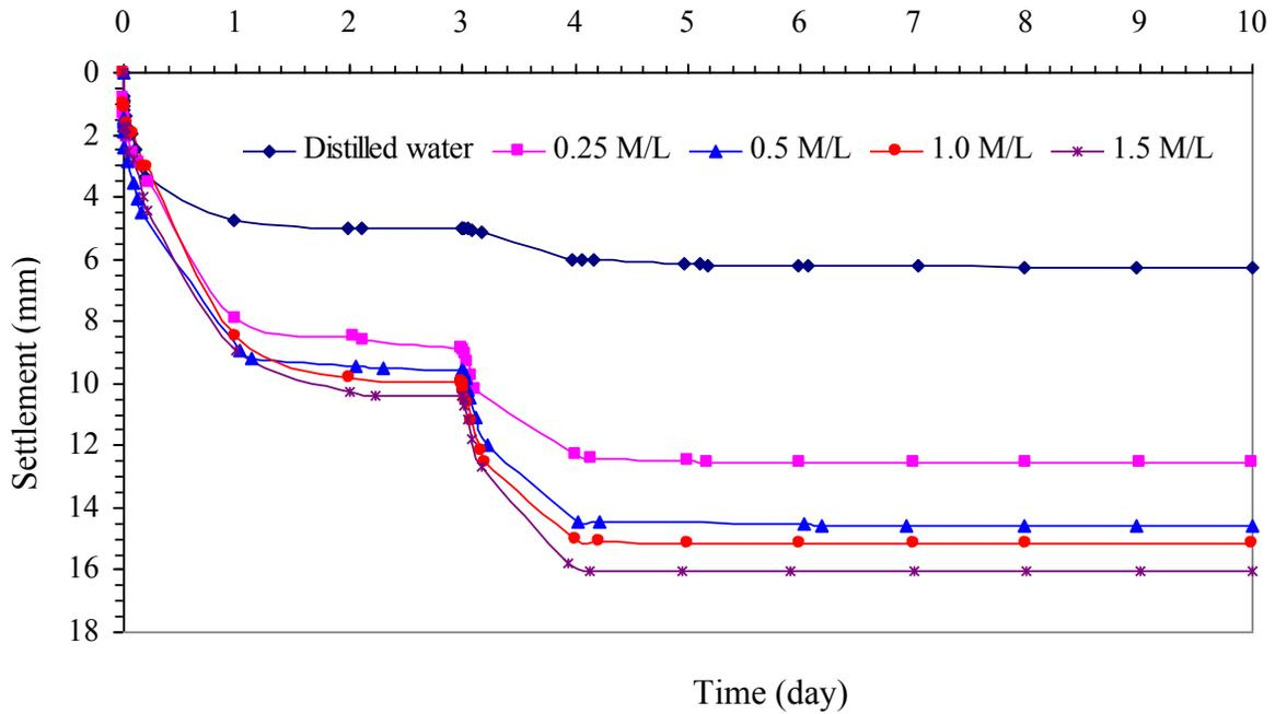
**Fig.8.** Variation of settlement with time for different fluids
