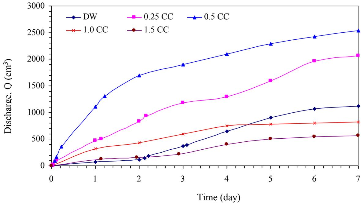
**Fig.5.** Variations of discharge fluid from cathode with time. DW= Distilled water, CC= Calcium chloride
