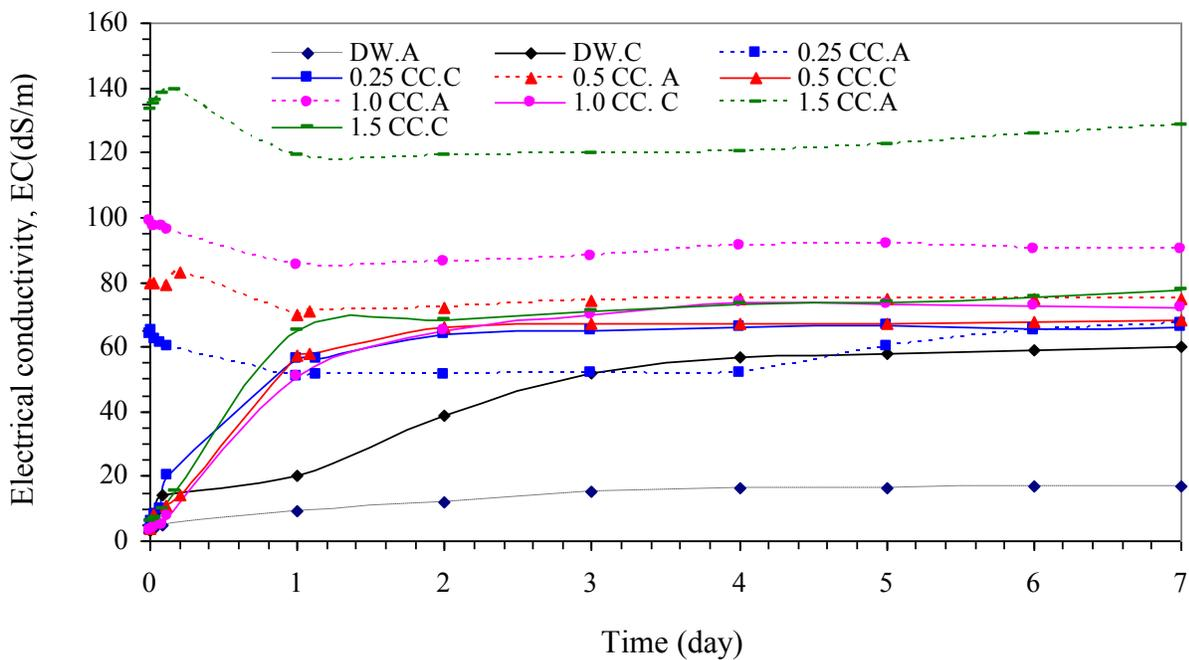
**Fig.4.** Variations of EC with time. DW=Distilled water, CC= Calcium chloride A=Anode, C= Cathode
