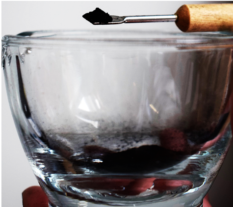
Figure 2.3: Image showing ground-up charcoal in a mortar and on a spoon type implement ready to be placed onto a resin block with square indentation on the surface of the block.
