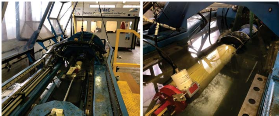
Figure 2: DMAc test rig with IMS installed (left); close-up of the IMS submerged in DMAc (right)
