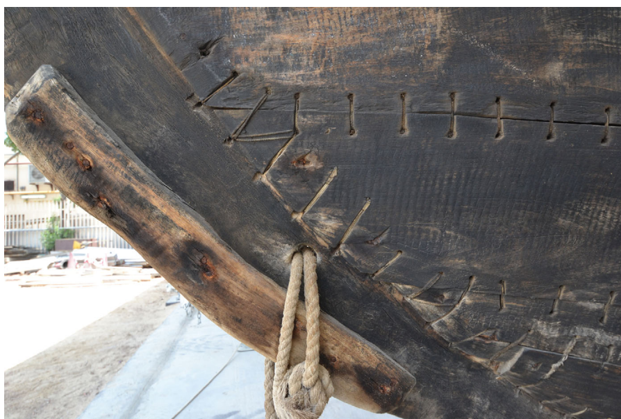
Figure 24. Painter holes occur in the stem and stern posts of kettuvallam B; the stern hole is also used to secure the steering oar. The two short timbers nailed on either side of the post are probably intended to reinforce the posts. (Image: Alessandro Ghidoni).
