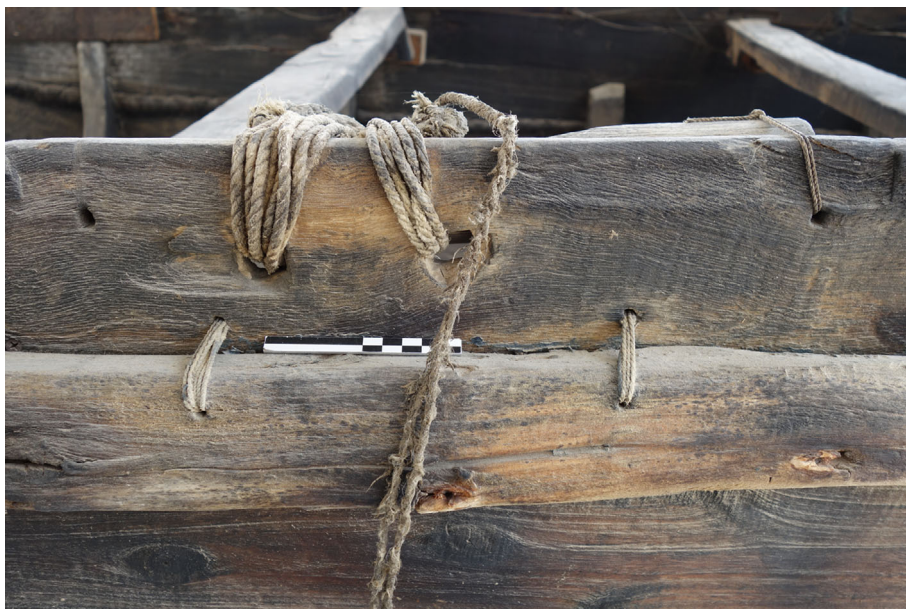
Figure 26. A rubbing strake nailed and lashed to the outer face of the sheer strake of kettuvallam B. (Image: Chiara Zazzaro).
