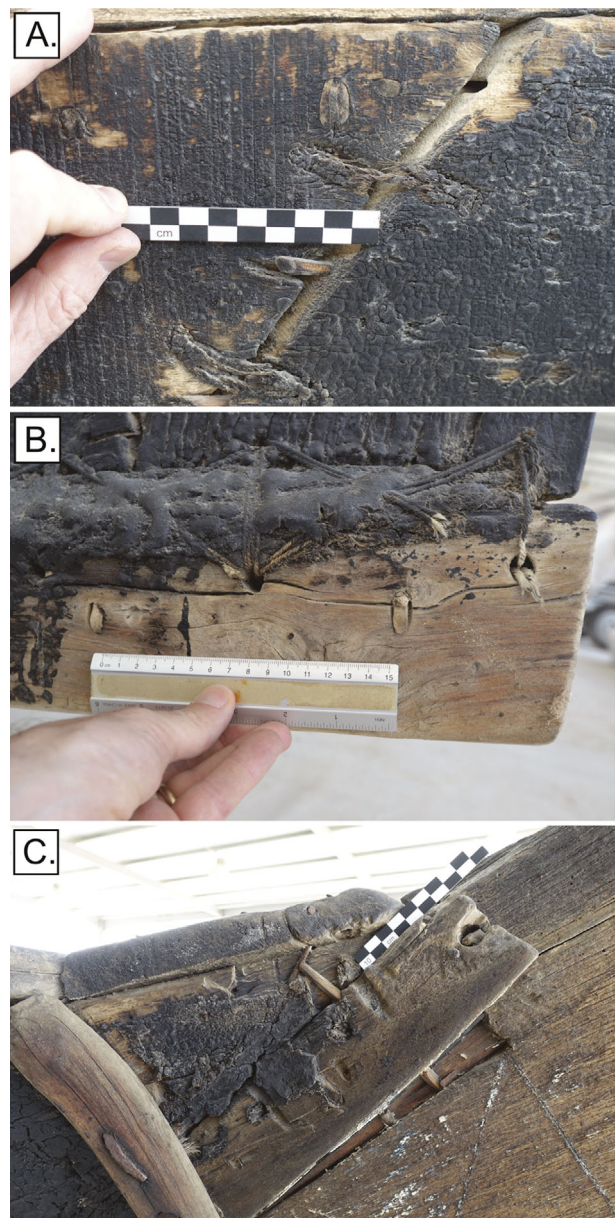
Figure 20. Oblique dowels used on the QM baggāras : A) securing a planking scarf joint on baggāra 1; B) fixing the fashīn to the keel, also on baggāra 1; C) fixing the ‘false’ stem and prow timber on baggāra 2. (Images: John P. Cooper, Alessandro Ghidoni).
