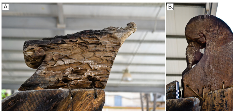
Figure 23. Decorative carved finials sewn to the posts of kettuvallam B. (Images: Alessandro Ghidoni, Chiara Zazzaro).
