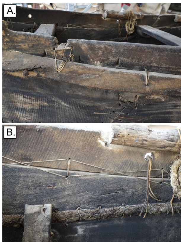
Figure 30. The wash strake and rubbing strake fastened to the sheer strake with stitching but no wadding on kettuvallam B: A) outboard, the vertical stitches act as lashings threaded through holes along the rubbing strake; B) the inboard view. (Images: Alessandro Ghidoni, Chiara Zazzaro).
